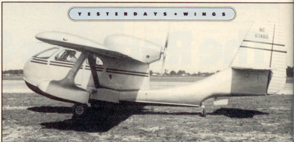
This view of a production RC-3 shows how the special long-shaft, 215-hp Franklin engine was built onto the cabin instead of being mounted on struts as on most pusher flying boats and amphibians.
