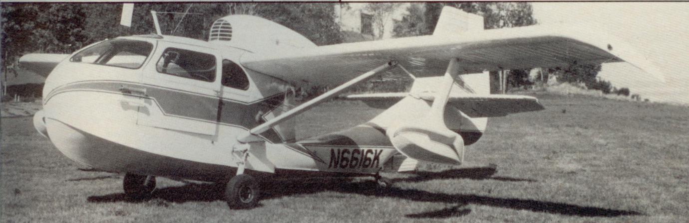
Although primarily a private-owner aircraft, the Seabee occasionally was used in commercial operations (top photograph). To enable the Seabee to carry extra paying passengers, the company would remove the amphibian's landing gear; the aircraft then operated only as a flying boat. The curved-down booster wing tips (directly above) were a popular modification to Seabees because they cut down on wing-tip vortex drag and increased wingspan slightly.
